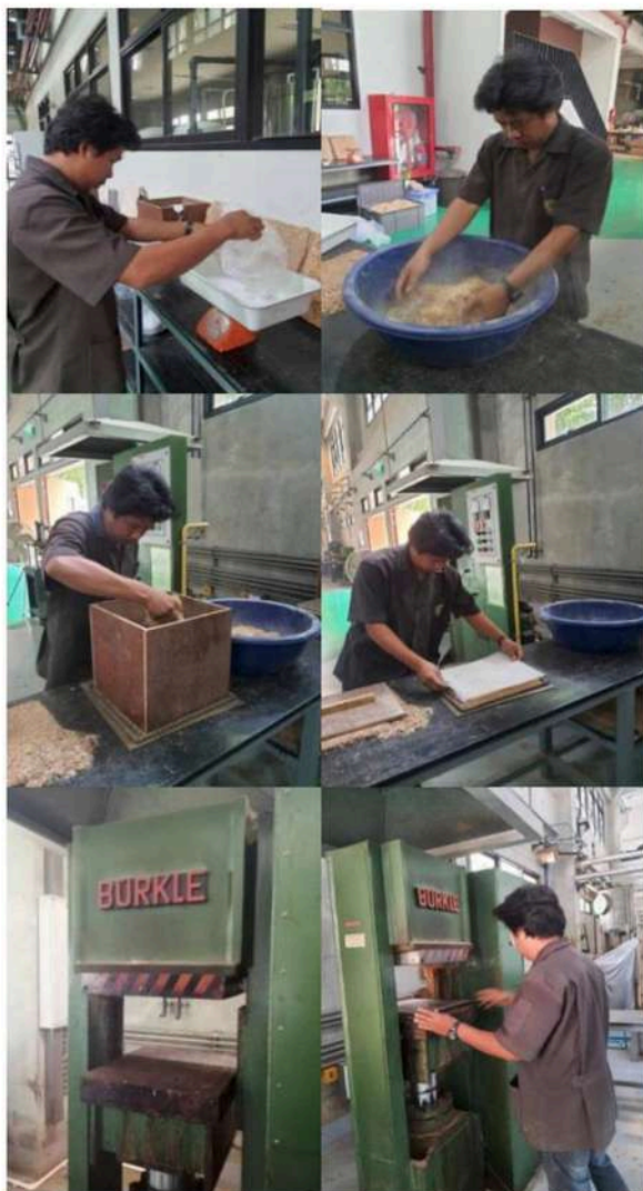
Fig. 3 Mixing particles of Giant Mimosa and other materials (by ratio) then forming the board and pressing it under appropriate pressure of 35\text{kg/cm}^2 and temperature of 200^\circ\text{C} for around 10 minutes
