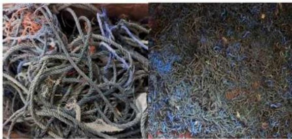
Cutting Nylon (Un-plasticised Polyvinyl chloride: uPVC) from fishing nets into small pieces @ approx. 1-1.5 cm
